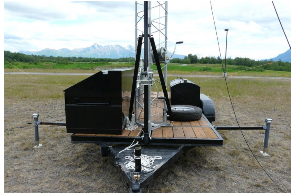
MAKE SURE IS ORIENTED NORTH LEVEL AND ALL OUT RIGGERS OUT AND SECURE
