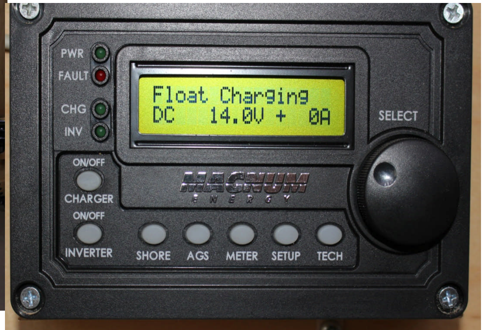
Make sure charger is on after connecting Outside AC power
