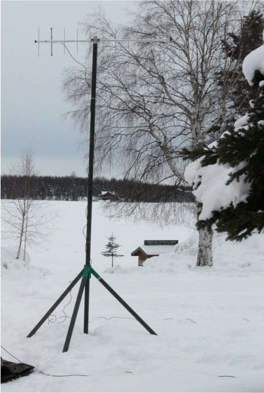
Camo Pole/golf bank mast setup
